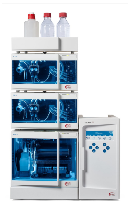
Figure 3. The ALEXYS Aminoglycosides Analyzer is the recommended instrument configuration for the analysis of Spectinomycin. It consists of an ALEXYS base system and an additional pump for post column NaOH addition.
